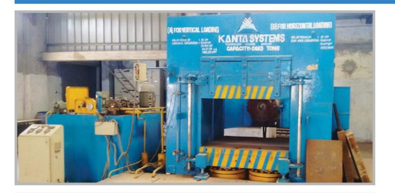
**F**ollowing strict quality standards, we maintain state-of-the-art testing facilities including a well-equipped laboratory and test Press of 2463 Tons – Vertical and 500 Tons – Horizontal load capacities.
