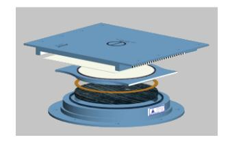
FREE BEARING allows rotation, longitudinal movement & transverse movements. The main components of a free bearing are the same as those of a fixed bearing, but are able to provide two-direction movements. Its piston top is attached with a PTFE coated sheet and supports a steel upper sliding plate, which needs a polished smooth stainless plate adhered to the contact surface between PTFE and the sliding plate to promote sliding movement.
