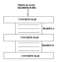
8.3 Bearing shall be preloaded up to 20 MPa and shall be allowed to retain for 10 minutes and then to be unloaded to initial position.
